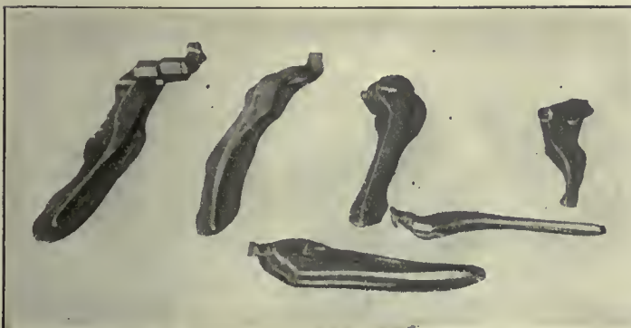
FIG. 3. DROP-FORGED WRENCH PARTS
